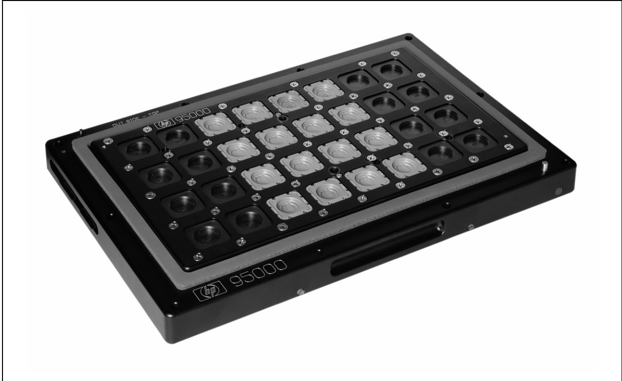
Figure-9 Contactors (16x) and Loadboard Assembly
